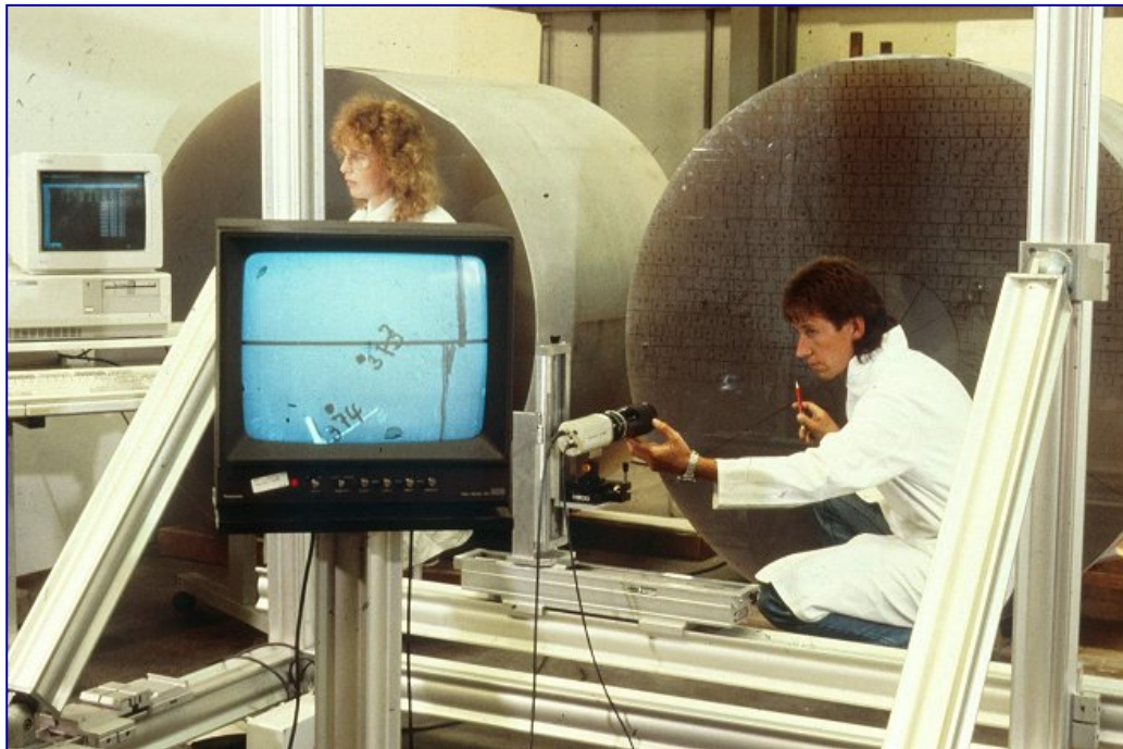
Figure 4: Focal scanning of large thickness ZERODUR® boules with an IR sensitive CCD camera (for AXAF/ Chandra).
