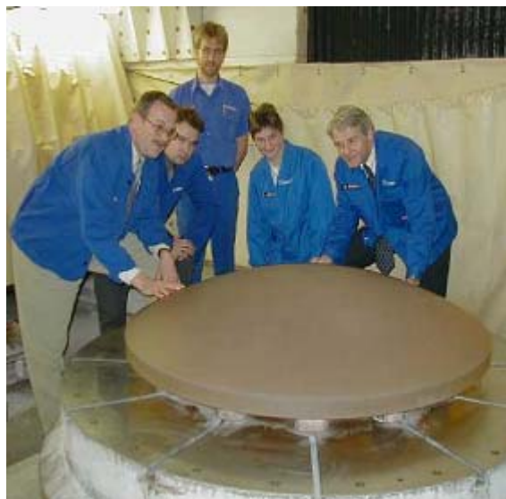
Figure 1: 1.33 m diameter testing lens for the secondary mirror of GRANTECAN
