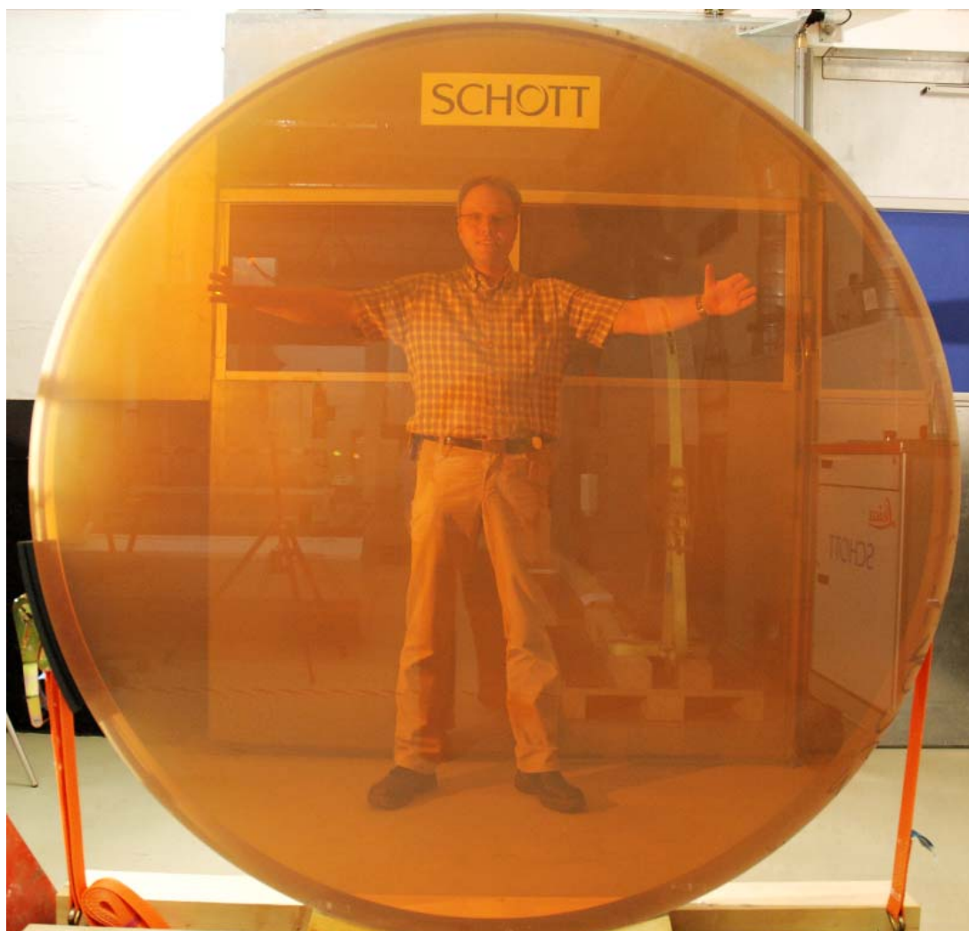
Figure 7: 1.53 m diameter and 176 mm thick, 819 kg heavy ZERODUR® blank with optical standard grade striae quality and excellent bubbles and inclusion quality.
